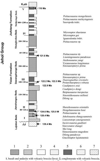
3, sandstone and conglomerate; 4, tuffaceous sandstone and tuff; 5, shale and tuff; 6, silt and silty mudstone; 7, subvolcanic rock
