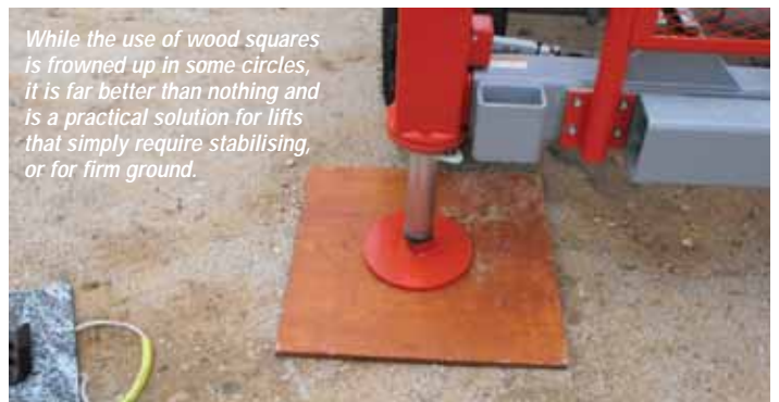
This neat little mat is used with van mount stabilisers rather than outriggers
