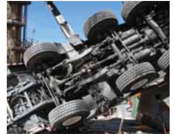
In this accident a two shift scenario caught the operator unaware that his rear outriggers had been left in the retracted position
