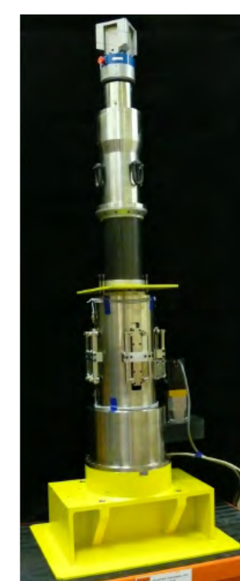
Full size, fully functional prototype mirror hardpoint being testing at NOAO
