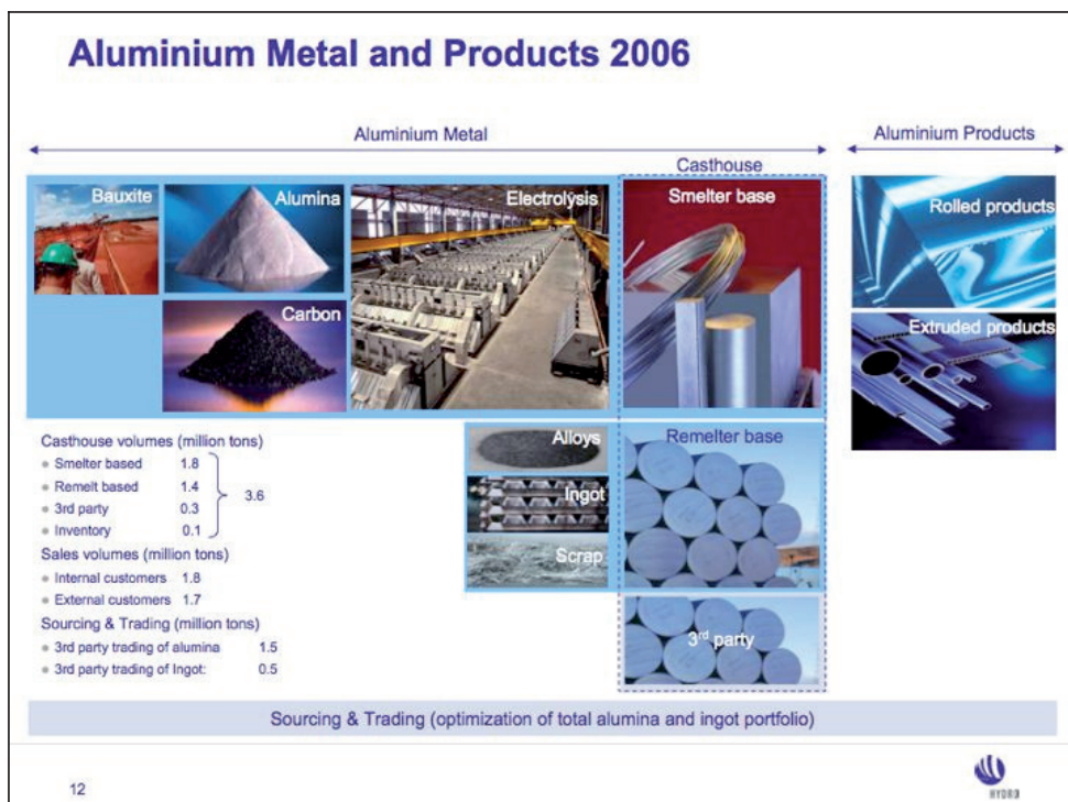
Figure 1. Hydro as “an integrated aluminium company”. The complete value chain, with outline of main production activities and volumes in different segments (Source: Hydro “Investor Presentation”, July 2007).
