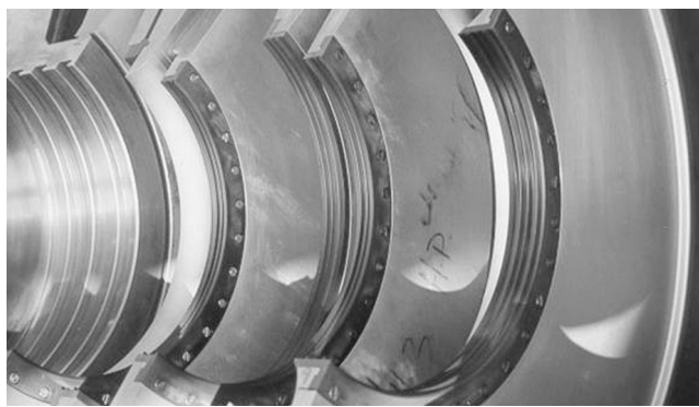
Figure 23. Photograph of TORLON® Seals Installed in Propylene Compressor. (Note the axially bolted construction.)
