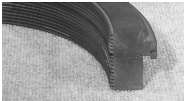
Figure 15. Picture of Broken Balance Piston Seal.
