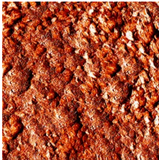
Figure 6.8 A 2 μm x 2 μm in situ AFM image of annealed osmium silicide grown by the regular method showing an overall smoother surface and structure in comparison with the as-grown of the same method. Annealing of films grown by the regular method leads to an overall better quality film.
