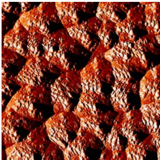
Figure 6.5 A 2\ \mu\text{m} \times 2\ \mu\text{m} in situ STM image of as-grown osmium silicide grown by the template method showing hillock-like surface and structure with uniformity for the textured grains.
