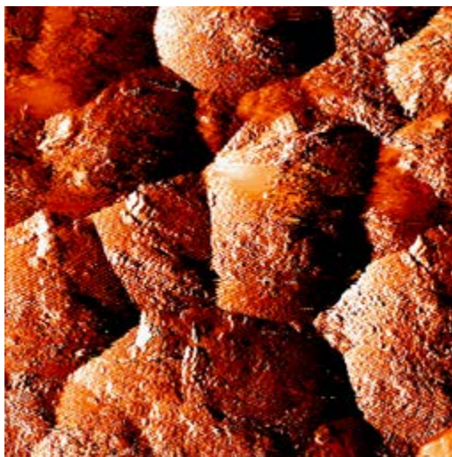
Figure 5.7 A 2 \mu\text{m} \times 2 \mu\text{m} STM image of as-grown diruthenium trisilicide film showing textured grains of around 0.5 \mu\text{m} in size.
