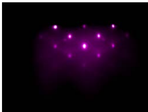
Figure 6.1 RHEED pattern of as-grown osmium silicide grown by the template method showing 3d-growth and great similarity to that of \text{Ru}_2\text{Si}_3 . Chapter 1 mentions that \text{Ru}_2\text{Si}_3 and \text{Os}_2\text{Si}_3 are isostructural 2 .
