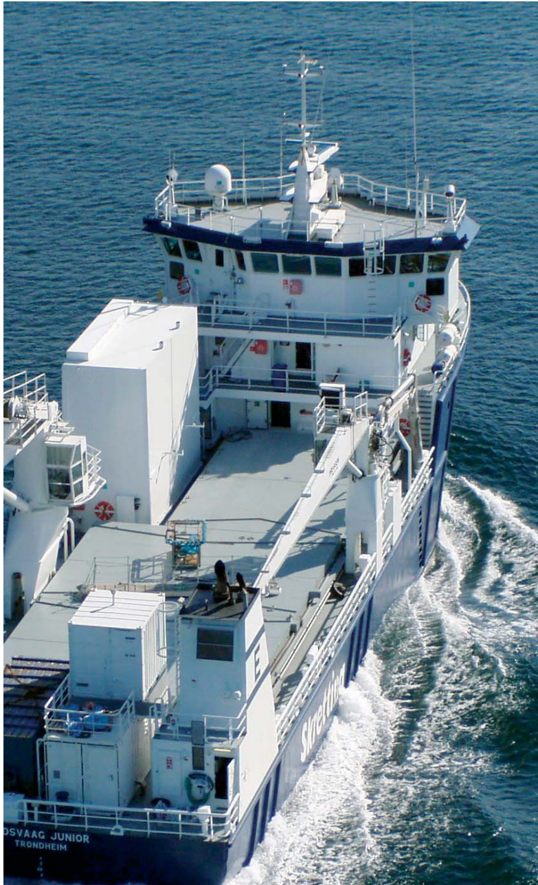
The coastal hull market is large and diversified. The Eidsvaag Junior is a purposebuilt fish fodder carrier for the fishfarming industry.
