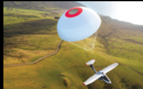
Complete airplane parachute
