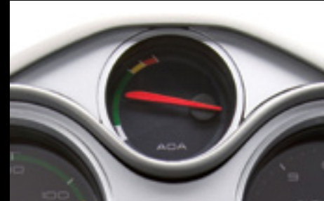
Angle of attack indicator
