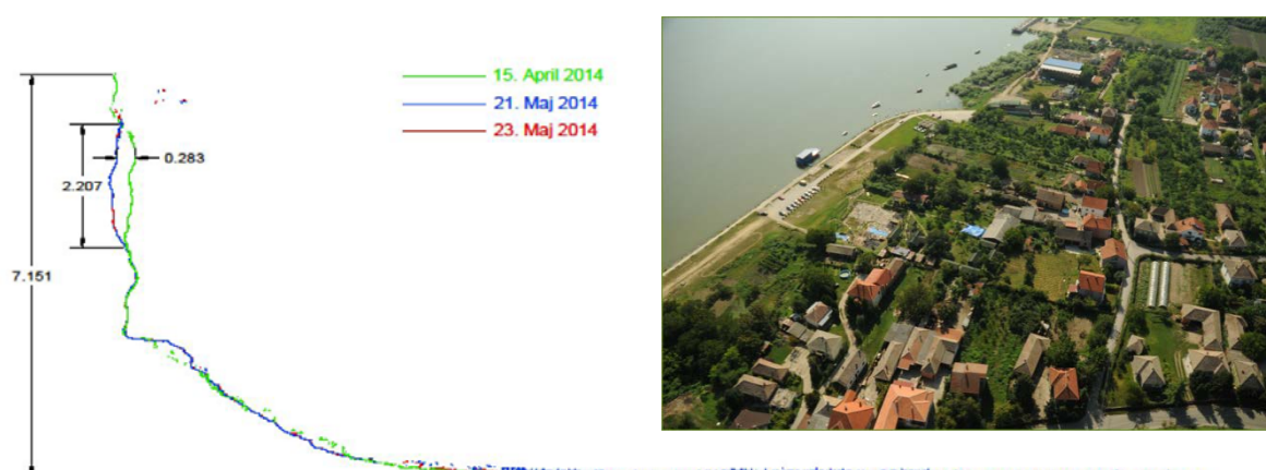
Figure 1-36. Profile section of the archaeological site of Vinča, with the changes recorded before and after the flooding period
