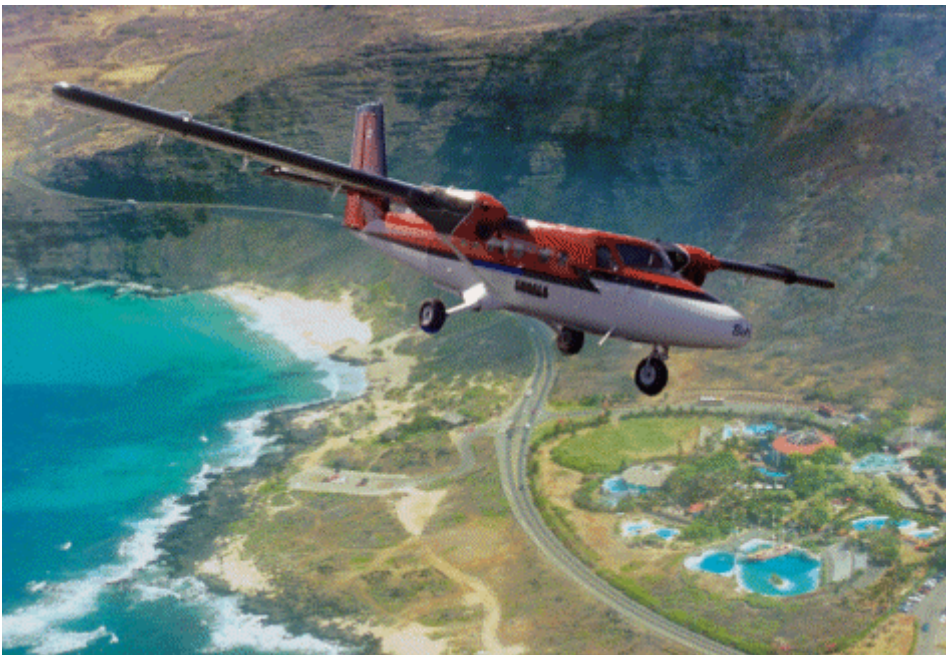
Figure 5: SHOALS lidar bathymeter in Kenn Borek Twin Otter over Hawaii.
