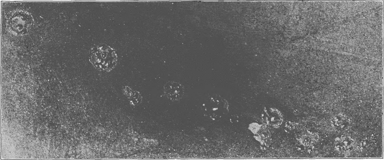
FIGURE 4.—Metal projected from a hot electrode globule to a cold electrically insulated plate when an incandescent electrode is moved at a speed of four feet per second over the surface of the plate. The photograph shows only a small portion of the projected metal, the remainder being scattered beyond the region photographed, or having become detached from the plate together with some of the flaky oxidized surface. The magnification is 8.2 diameters.
