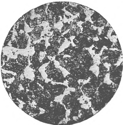
FIGURE 2.—Steel containing 0.37% carbon, light portion—Ferrite; dark portion—Pearlite; magnified 500 diameters.
