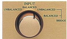
Switchable bridged operation mode
