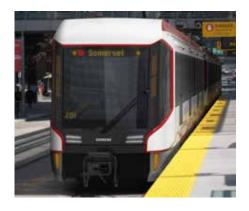
S200; a steel carbody construction, fully bidirectional, single articulated, high-floor vehicle – ideal for high platform operation and built in North America.
