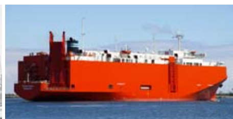
TAKARA: In 1977/78 the ship was rebuilt from bulk to ro-ro car carrier.
