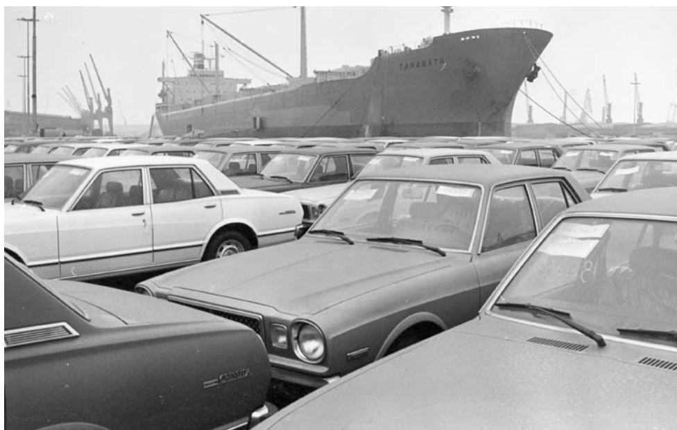
TANABATA: The former bulk ship was converted to ro-ro car carrier in 1977/78.
