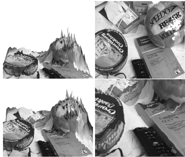
Figure 13. Some views of the reconstruction obtained from the desk image pair. The inaccuracy at the top of the volleyball is due to the depth ambiguity at the epipole.
