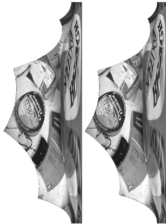
Figure 10. Rectified pair of images of the desk. It can be verified visually that corresponding points are located on corresponding image rows. The right side of the images corresponds to the epipole.
