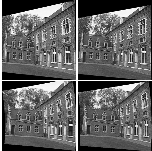
Figure 8. Rectified image pair for both methods: standard homography based method (top), new method (bottom).
