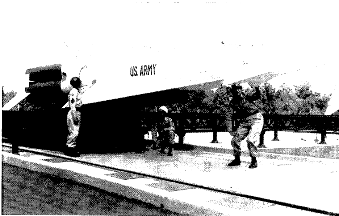
A solid-fuel Nike Hercules missile rests on its elevator-mounted launcher. The four dark colored solid-fuel boosters are clustered together just forward of the tail.
