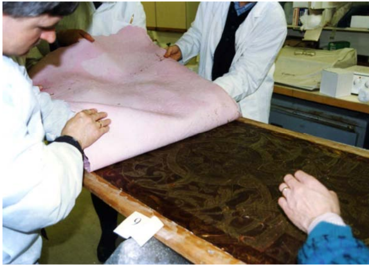
Fig.3. A flexible silicone rubber mould is taken from the original leather to produce a negative impression of the rich and intricate relief pattern embossed in the leather.
