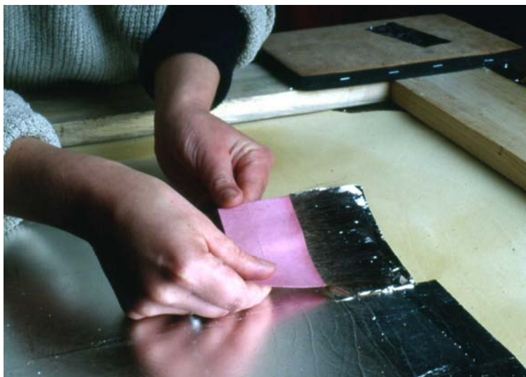
Fig. 5. The vegetable tanned calf leather stretched on the wooden frame, moistened, and coated with a thin layer of the parchment glue, is covered with leaves of metallic silver.
