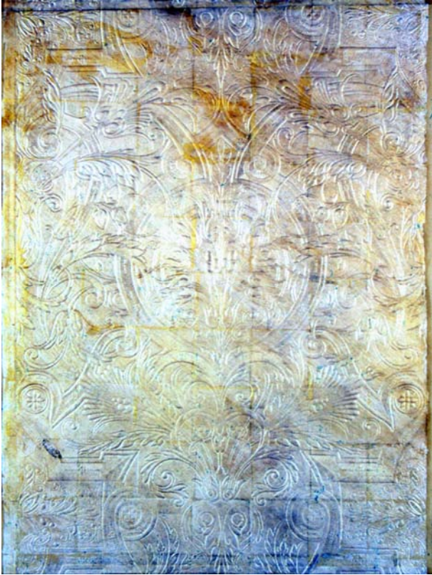
Fig. 7. The silvered and varnished leather with a relief produced from the moulding plate under the pressure.
