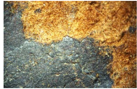
Fig. 6. Detail. On the left hand side the dark flesh side of the leather is covered with a wax layer. On the right hand side the lighter collagen fibres are seen after removing the wax. Magnification 12.5.
