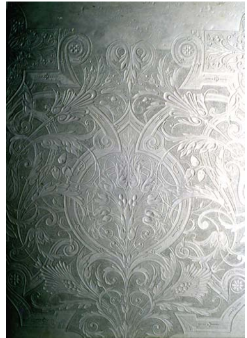
Fig. 4. Plaster of Paris was cast into the silicone rubber mould and the positive impression obtained was re-worked, corrected and made complete. This re-worked plaster cast served to produce the new moulding plate of epoxy resin reinforced with Duraluminum powder, shown in the illustration. The material provided necessary high strength which could withstand high pressure during the leather embossing process.
