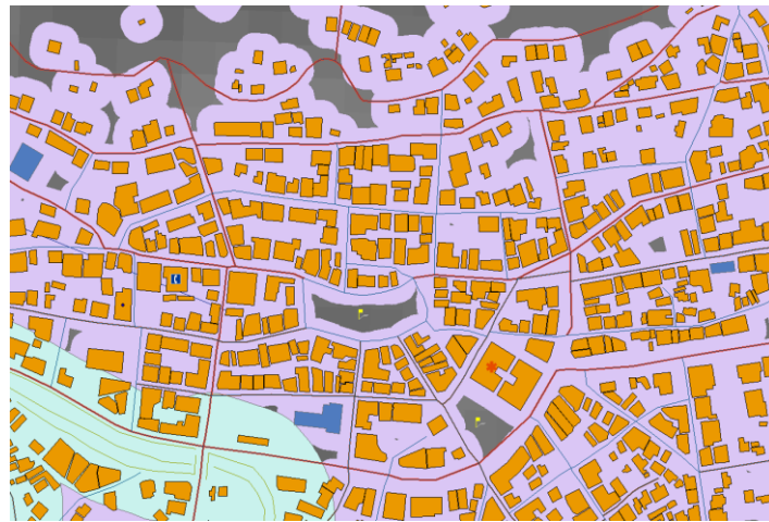
Fig. 5. Assembly areas (flagged) and emergency road network in the city of Grevena as determined with the use of GIS tools. Collapse buffer zones around existing buildings (purple color) and buffer zone alongside Grevenitis River (light blue color) can also be seen [23]
