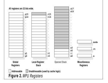
r14). Theses registers and the remaining register (r15) operate together as a stack cache. As a stack, they are used to hold subroutine return addresses and automatically nest local-register data. External local-register stack memory is addressed by register 1a.
