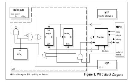
The interrupt controller (INTC) allows multiple external or internal requests to gain, in an orderly and prioritized manner, the attention of the MPU. It supports up to eight prioritized interrupt requests from twenty-four sources. Interrupts are received from the bit inputs through ioin, from I/O-channel transfers, or from the IOP interrupt instruction int.
