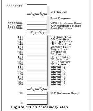
Associated with each of the eight interrupt requests is an interrupt service routine (ISR) executable-code vector located in external memory. See Figure 10. A single ISR executable-code vector for a given interrupt request is used for all requests on that interrupt. It is programmed to contain executable code, typically a branch to the ISR. When more than one source is possible, the current source might be determined by examining associated bits in ioin, ioie, iodmae and the global registers.
