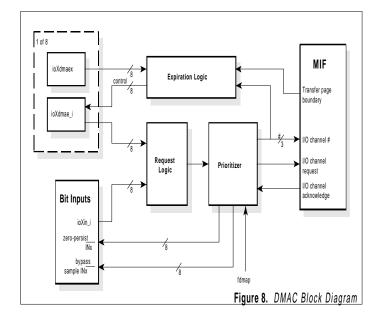
The Direct Memory Access Controller (DMAC) allows I/O devices to transfer data to and from system memory without the intervention of the MPU. It supports eight I/O channels prioritized from eight separate sources. Direct memory access (DMA) requests are received from the bit inputs through ioin. DMA and MPU bus request priorities are either fixed, which allows higher-priority requests to block lower-priority requests, or revolving, which prevents higher-priority requests.
