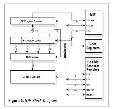
The Input-Output Processor (IOP) is a special-purpose processing unit that executes instructions to transfer data between devices and memory,
