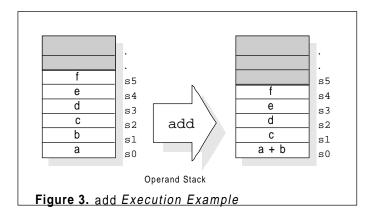
Most ALU operations behave similarly, using two source operands and returning one result operand to the operand stack. A few ALU operations use one source operand and return one result operand to the operand stack. Some ALU and other operations also require a nonstack register, and a very few do not use the operand stack at all.
