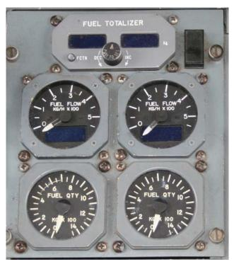
Figure 3: Fuel management panel in the cockpit centre console instrument group.
