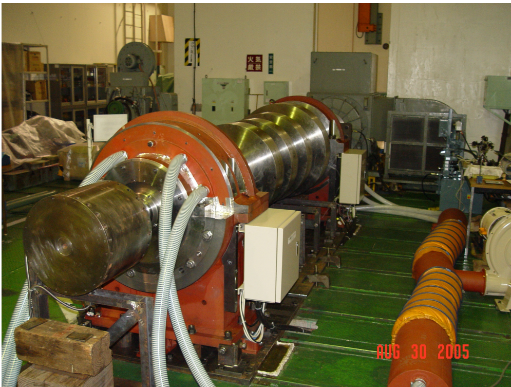
Fig 11. MB rotor test rig of 1/3 of the GTHTR300C full scale
