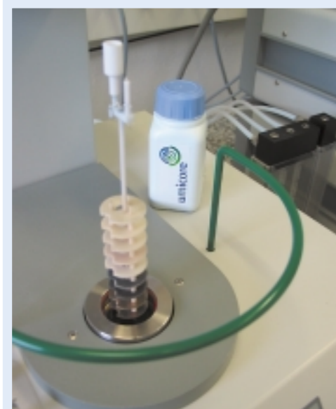
Placing a sample in a ceramic crucible on the measuring head.
