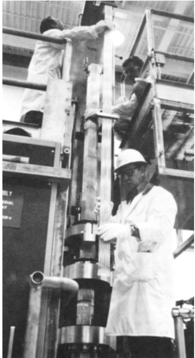
FFTF technicians working on a fuel assembly. Each fuel pin is less than a quarter-inch in diameter and about 8 feet long. The fuel pins are gathered into 217-pin assemblies, like the one shown here, which are housed in hexagonally shaped ducts in the reactor core.
