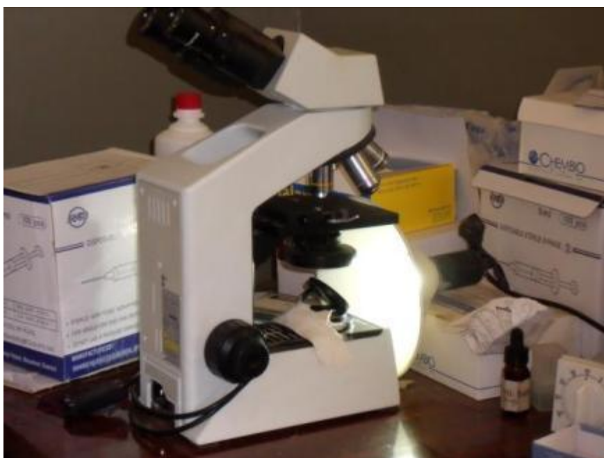
Picture 36: The microscope using a solar lamp as light source.
