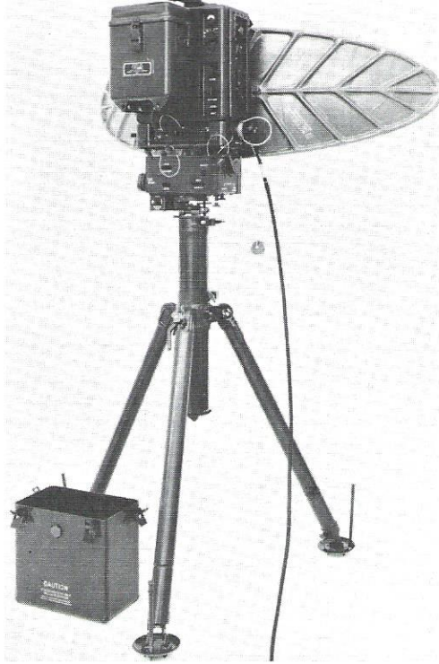
The basic radar unit weighs 56 lb and requires only 42 watts of power. Used alone the basic radar provides aural surveillance. The scanning head of the AN/PPS-5 is engineered to be inaudible at a distance of 15 metres when in operation.
