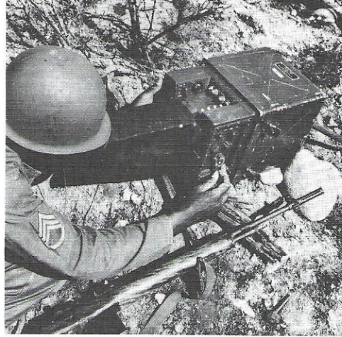
The remote unit of the radar in operation in the field. With the two visual displays the operator can maintain surveillance on multiple targets within the scanned sector up to a range of 10,000 metres.
