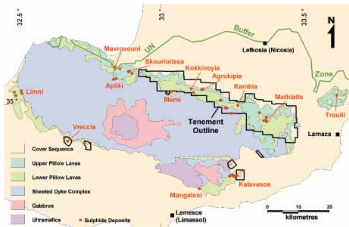
Figure 4: Geological map of Troodos Complex, showing the principal geological units described below, as well as the locations of the EMED Permit and Application Tenement areas and most of the historic deposits. Note that the Skouriotissa mining operation comprised three separate deposits (Phoukasa, Phoenix and Three Hills).
