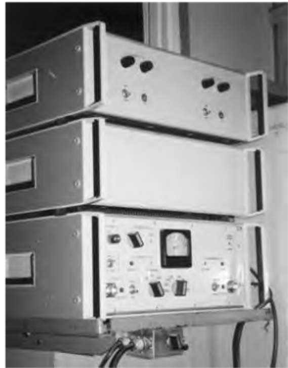
MW jamming modulator "Zenit-M" at Sitkūnai radio center in Lithuania
