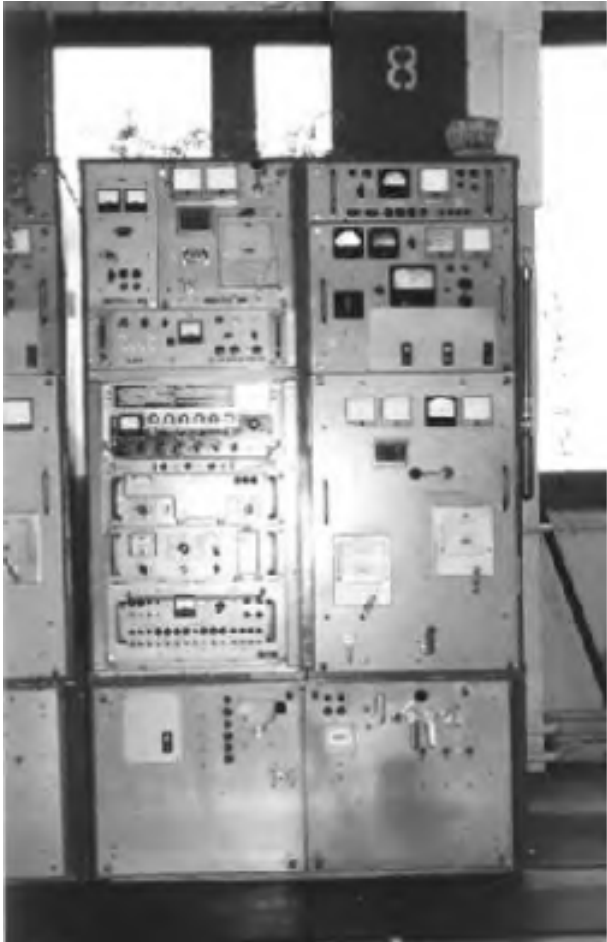
2.5/5 kW SW communications radio transmitters "Viaz-M2" (USSR), used at the local radio jamming stations in the late 70's and 80's.
