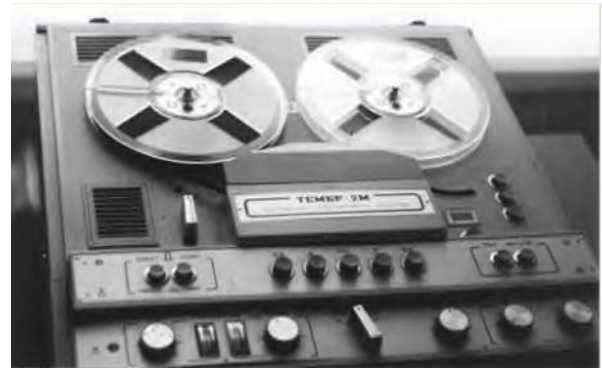
Tape-decks "Tembr" for playback of the "speech-like" audio signal, used for jamming in the USSR in 1976-1988.
