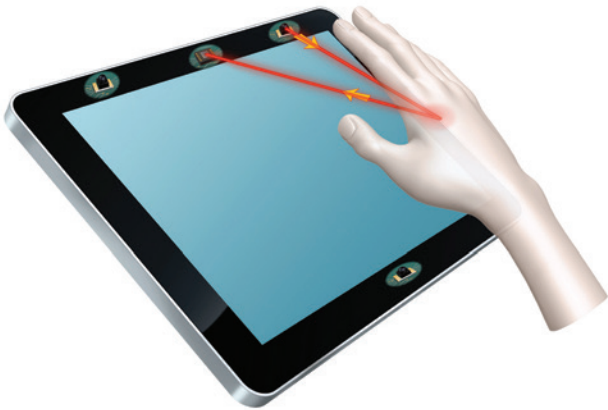
Proximity controls rely on IR emitters and receivers to gauge time-of-flight to register 3D hand position.
