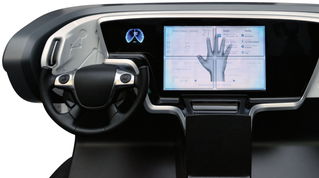
A “high-five” hand position with spread fingers commands the Horizon system without touching. (Visteon)
