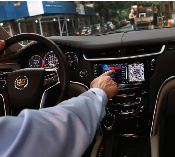
Cadillac's CUE touch-less control system uses infrared sensors to interpret hand gestures.
