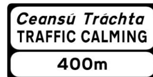
P 063: Traffic Calming Ahead
