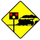
W 120 Level Crossing With Flashing Red Signals
