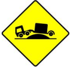
W 123 Risk of Grounding
