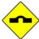
W 132 Humpback Bridge
