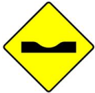
W 131 Road Depression
