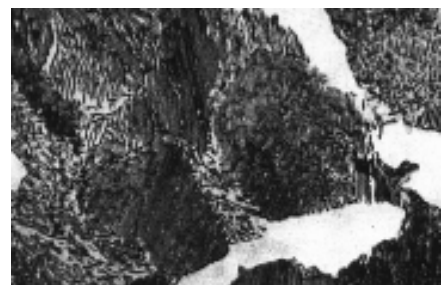
Fig. 6. Same as Fig. 5, normal pearlite. BF, 1000:1
