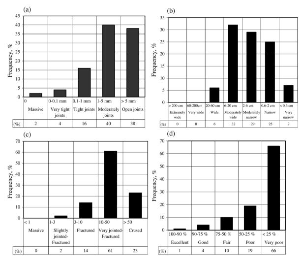
Fig. 4. Histograms showing percentage distribution and classification of basalt (a) based on fracture spacing (Deere, 1963), (b) distance between fractures (ISRM, 1981), (c) frequency of fractures in 1 m (ISRM, 1981) and based on RQD (Deere, 1963).
