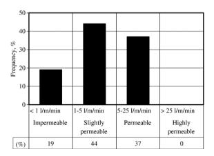
Fig. 6. Histograms showing percentage distribution and classification of basalt based on the Lugeon unit (Lugeon, 1933).
