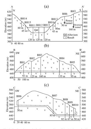
Fig. 3. Engineering geological cross-sections of the (a) dam axis, (b) diversion tunnel and (c) power tunnel.
