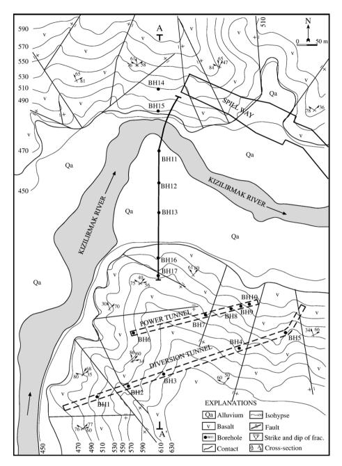
Fig. 2. Locations of the boreholes, main structures, and engineering geological map of the Obruk dam site.
