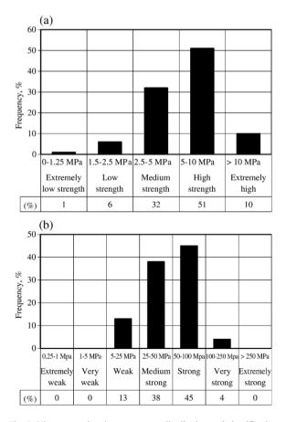
Fig. 5. Histograms showing percentage distribution and classification of basalt based on (a) point-load index (Deere and Miller, 1966), and uniaxial compressive strength (ISRM, 1981).
