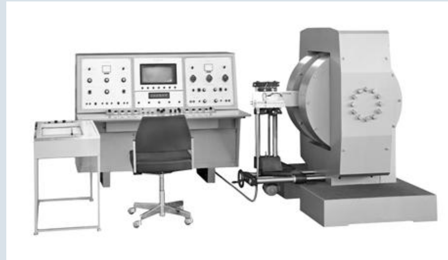
1967: HFX 90, the first fully transistorized NMR system, equipped with three independent channels
