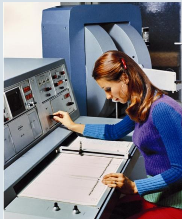
1971: WH 90, the first FT-only NMR Spectrometer
