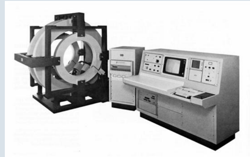
1983: One of the first whole body MRI tomographs with air coil magnet
