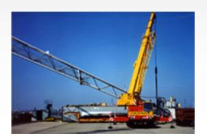
16ton MAN Travelling gantry Crane - Boom being assembled
