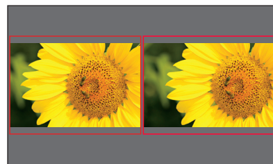
Phantom 65 Full Frame 4096 x 2440 pixels 51.20mm x 30.50mm 59.60mm diagonal
