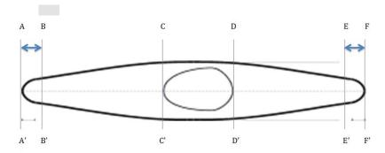
Section AA' to BB' - Front Impact Zone - measured to the point 100mm down the length of the kayak 100 mm minimum radius at any point on B-A-B'
