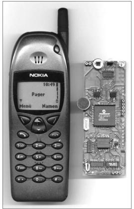
**Figure 2.** The sensor board and the enhanced mobile phone prototype.
