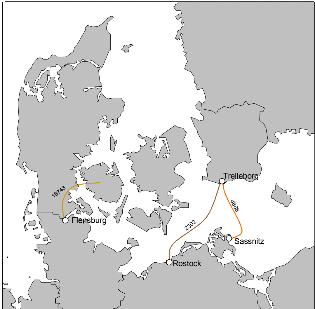
Figure 4.2.3: Number of freight trains/year by ferry line / routed via the Great Belt Reference Case A, 2015
