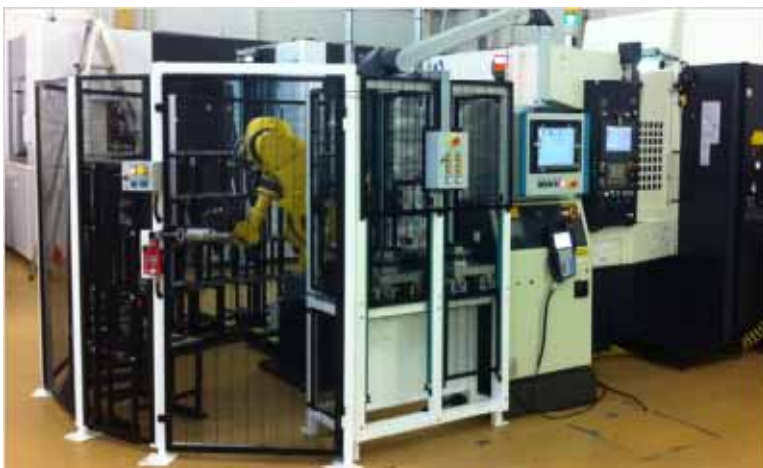
Makino grinding cell – a central target for resource holonification at GKN Aerospace Norway
