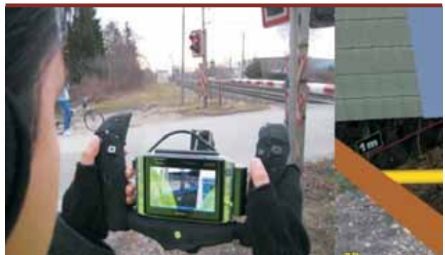
Augmented Reality in a Smart Phone connects the image of a natural environment with computed data from a GIS, perhaps showing an underground structure. This example is from project Vidente (2009).
