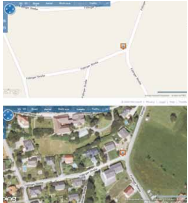
Example of a 2D street map and the vastly enriched information when superimposed by an orthophoto., This example is being taken from www.bing.com/maps .
