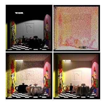
**Figure 13:** *Textured box with displacement-mapped teapot: direct illumination only, photon map, radiance estimates, and point-based global illumination.*
