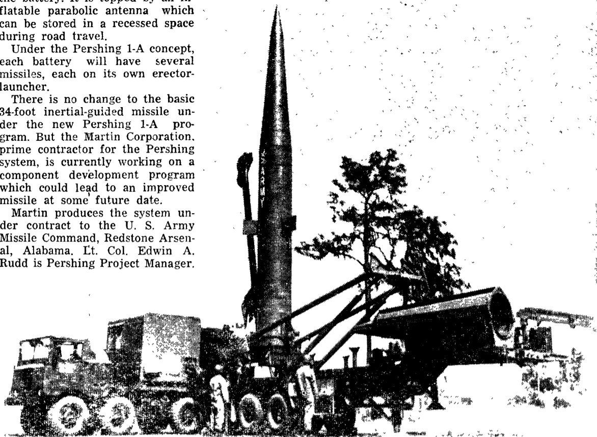
PERSHING ON WHEELS (Above) —The Army's highly mobile Pershing missile system is getting even faster movement, higher reliability and reduced maintenance cost through its new ground support equipment. Known as the Pershing 1-A, the system includes an improved erector-launcher with a tractor version of the M-656 five-ton cargo truck. The improved programmer station, radio terminal set and new firing battery control center each will be hauled on a M-656 cargo truck, a change from the tracked vehicles being used on the Pershing 1 which is already in the hands of troops. Supporting the development work on Pershing 1-A are Ford Motor Company for the trucks and Martin Marietta Corporation for the missile system.
