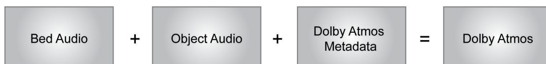
Figure 1-1 Simplified Dolby Atmos Block Diagram
