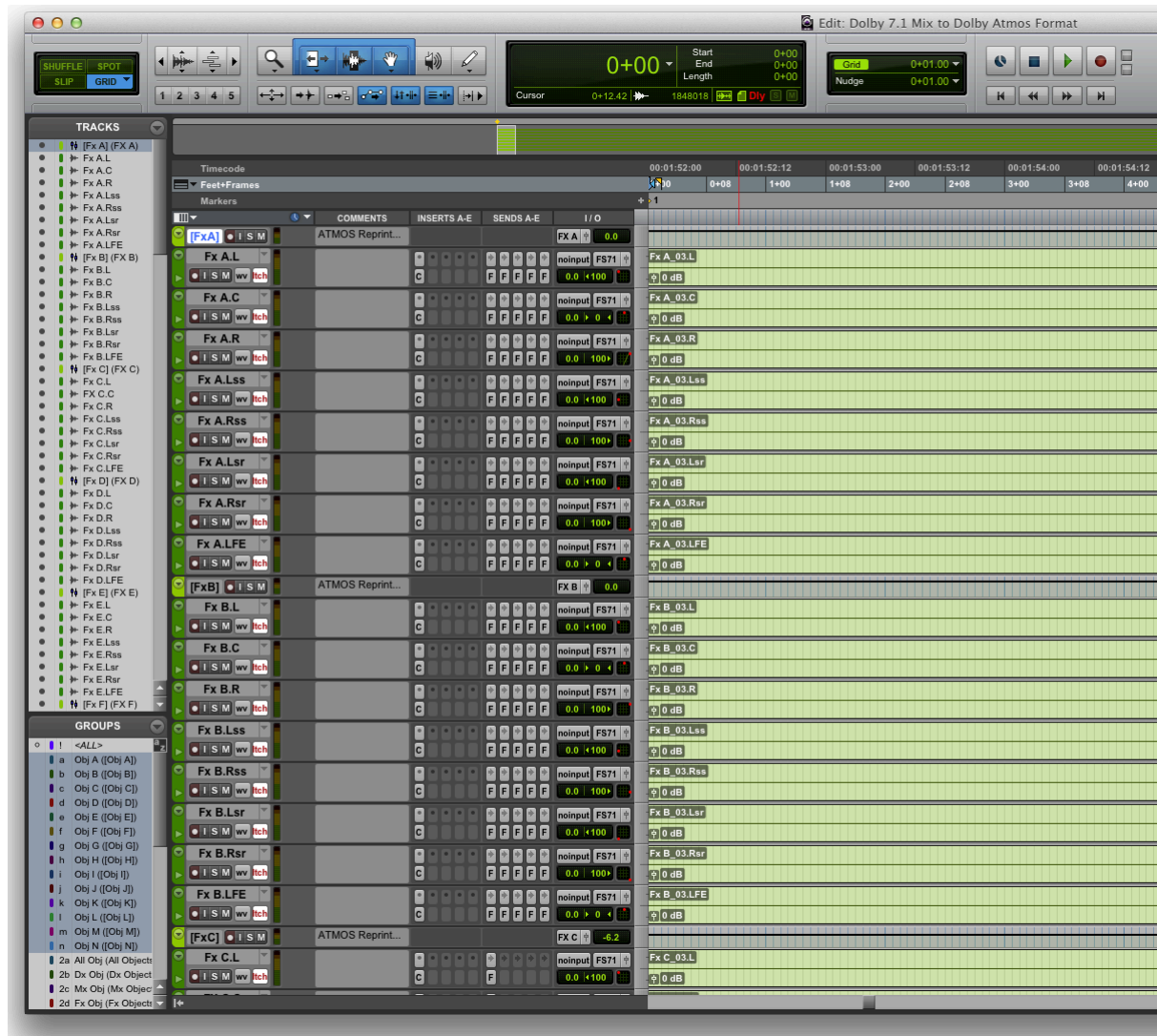
Figure 6-3 VCA Master Tracks Assigned to Each Effects and Foley Premix
