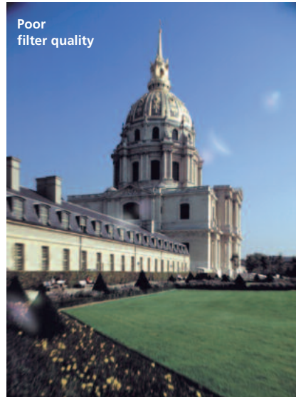
Low-quality filters reduce sharpness, generate reflections and contrast-reducing flare when shooting against the sun and they can cause vignetting.
