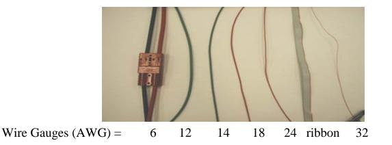
6 AWG (or larger diameter) must be used in battery-to-circuit breaker path
