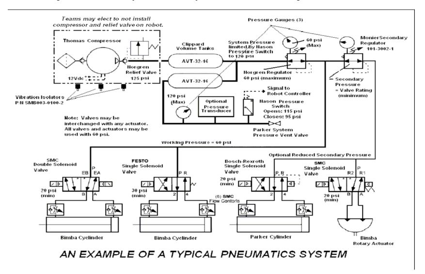
Pneumatics Diagram – If the robot uses pneumatics, the setup must be similar to the following.
