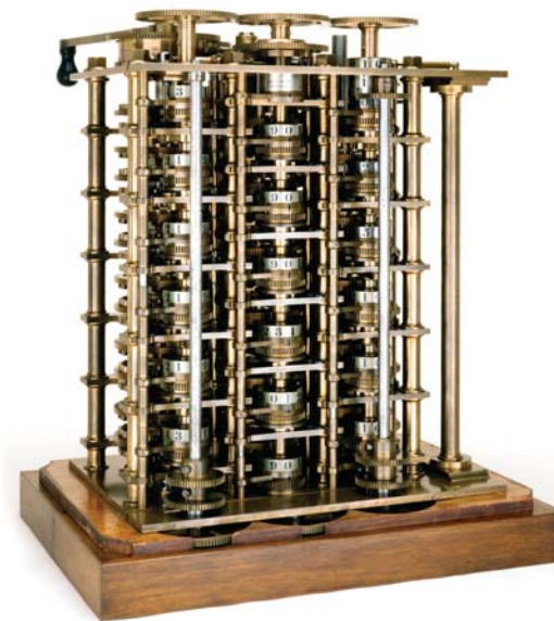
This portion of Babbage’s Difference Engine No. 1 was assembled in 1832 by his engineer, Joseph Clement, as a test. It consists of 2,000 parts and represents one-seventh of the complete engine.
