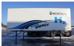
H 2 CYLINDER CONTAINER CAPACITY 235 or 390 KG/UNIT
