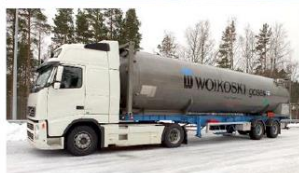
LIQUID HYDROGEN CONTAINER CAPACITY 2000 KG/UNIT
