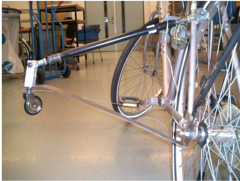
Figure 3.11: After one static test the sidewheels were plastically deformed to a large extent
