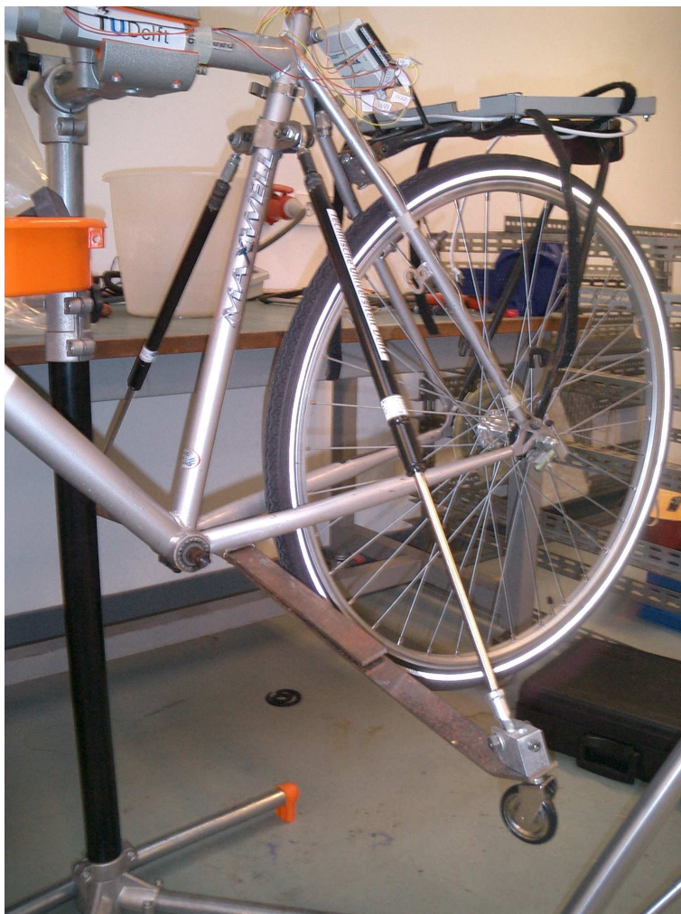
Figure 3.12: McPherson style side wheels
