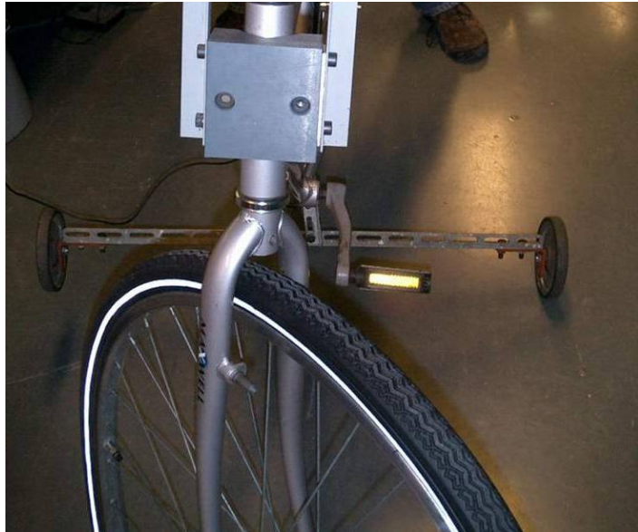
Figure 3.9: Stiffly added sidewheels
