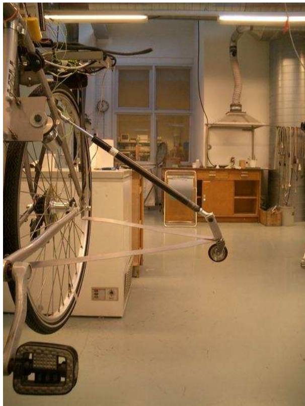
Figure 3.10: McPherson style side wheels
