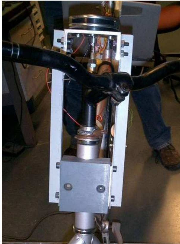
Figure 3.3: The steering angle sensor and bracket on the test bike
