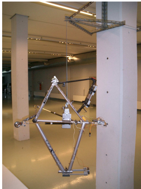
Figure 4.11: The rear frame clamped with its saddle tube in the horizontal position
