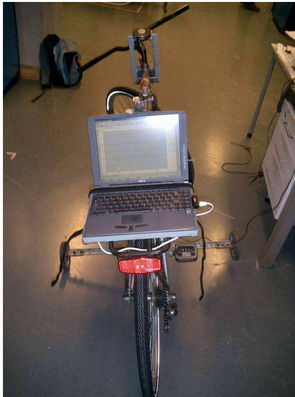
Figure 3.2: Laptop in the bracket on the rear rack
