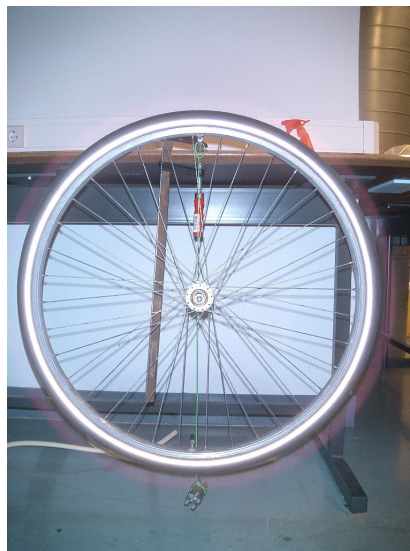
Figure 4.14: The front wheel during the compound pendulum experiment
