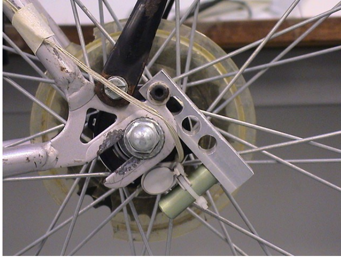
Figure 3.6: The pickup and its bracket
