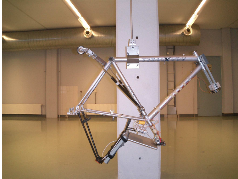
Figure 4.10: The rear frame clamped with its sloping tube in the horizontal position
