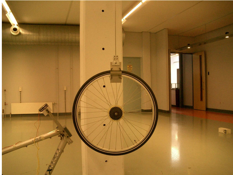
Figure 4.13: The rear wheel clamped in the torsion pendulum
