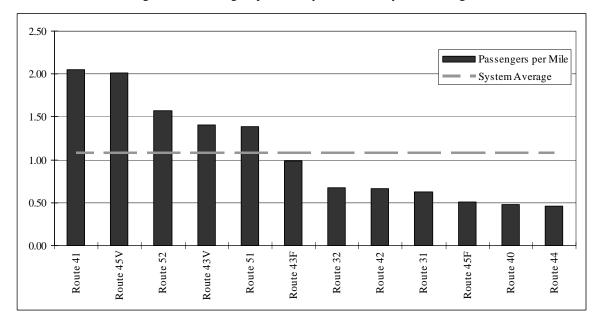
Figure 4-6: Passengers per Mile by Route with System Average
