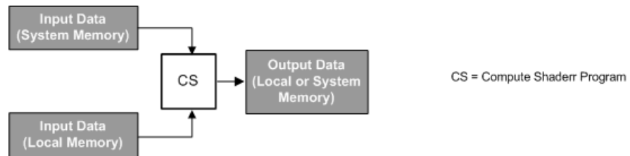
Figure 1.2 GCN Generation 3 Dataflow
