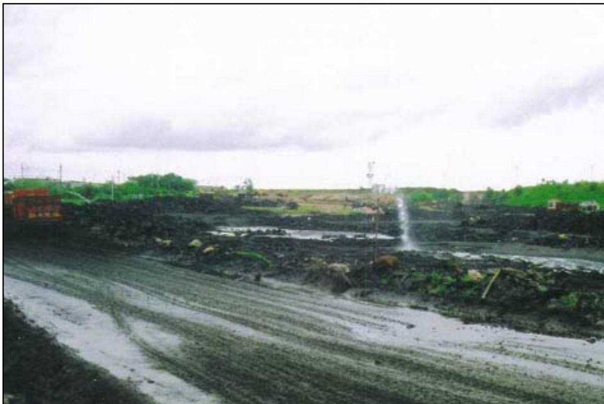
Fixed sprinklers to minimise air pollution at coal mine at Telwasa, Chandrapur
